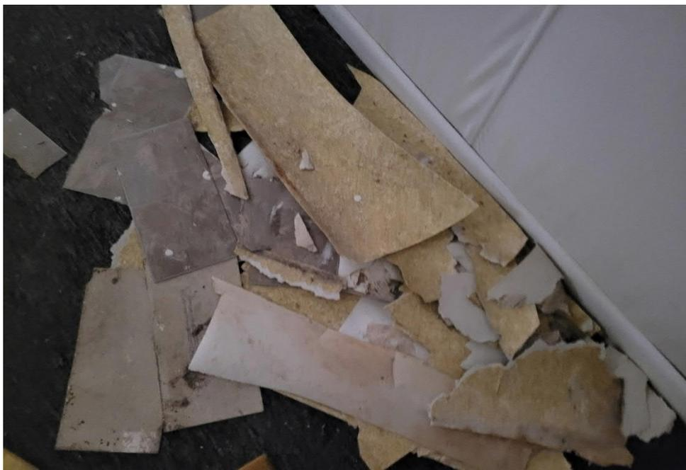
**Photo 8:** View of positive vinyl sheet flooring debris pile in building 211 1<sup>st</sup> floor west side office located in middle room and under carpet and shower.
