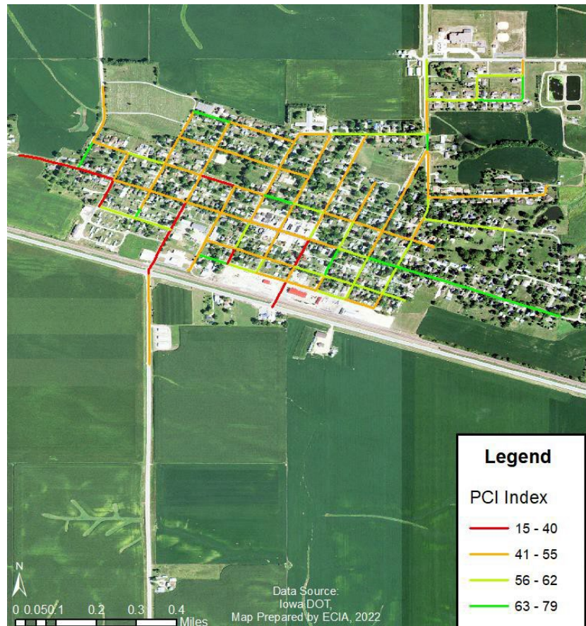
Figure 9. Pavement Condition Index, Mechanicsville
